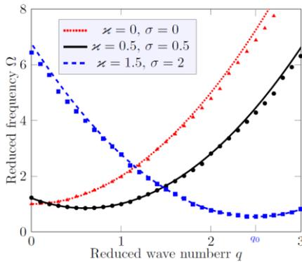
Fig. 3. Dispersion law of spinwave spectrum of the helix wire with easy-tangential anisotropy. Symbols correspond to simulation data and lines correspond to formula (21).
