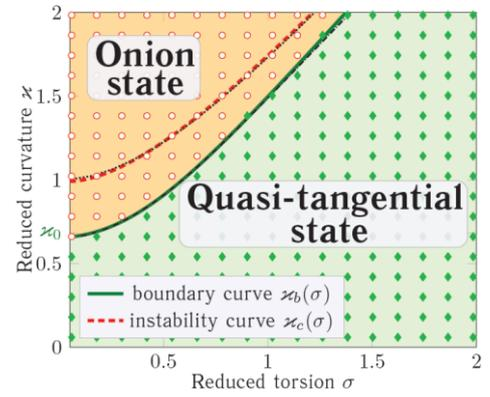
Fig. 2. Phase diagram of equilibrium magnetization states for helix wire with easy-tangential anisotropy. Symbols correspond to simulation data: green diamonds to quasi-tangential states and open circles to the onion ones.
