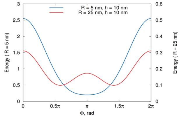
Fig. 3. Energy as a function of angular parameter  $\Phi$  for spherical shell with thickness 10 nm and different radii.
