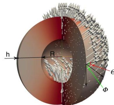
Fig. 1. Schematic of the spherical shell. White arrows correspond to the magnetic distribution.
