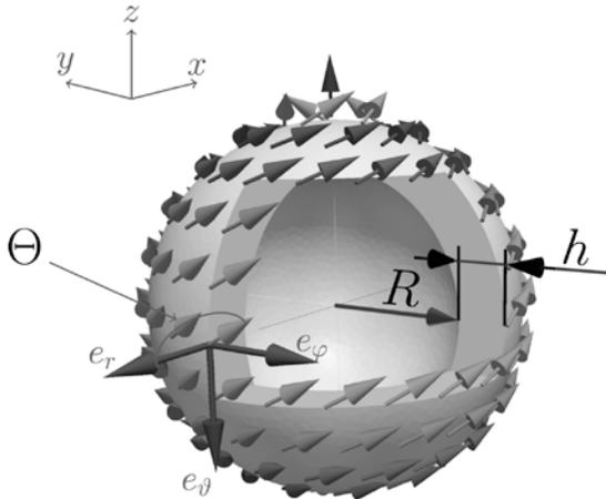
Fig. 1. Schematic of the spherical shell. Arrows correspond to the magnetic distribution.
