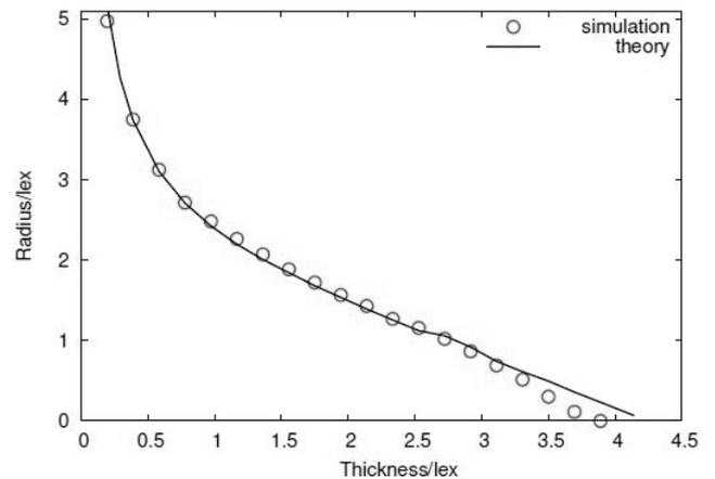
Fig 2. Normalized critical radius vs normalized thickness of spherical shell. Circles correspond to the simulation data and solid line shows theoretical values.
