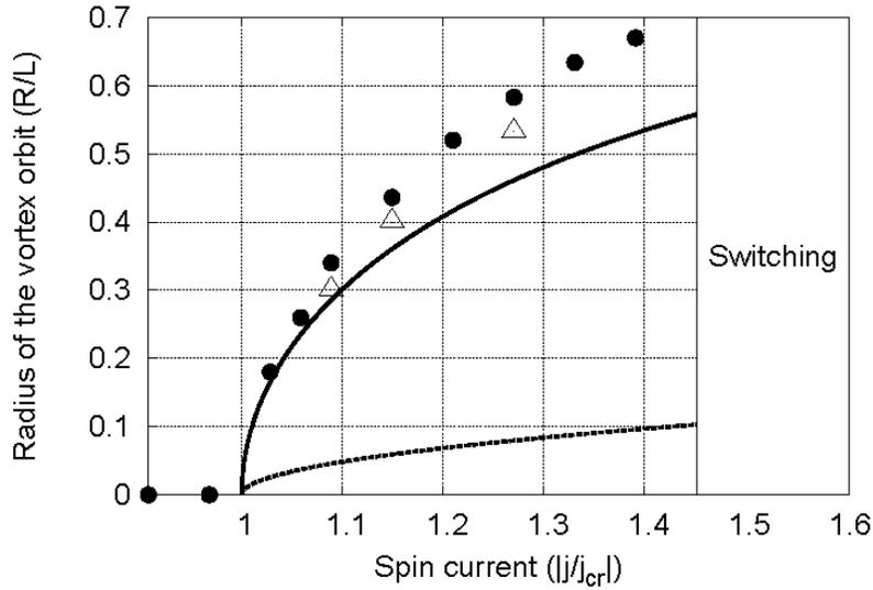
**Figure 4.** Radius of the vortex for the disk with  $2L = 50a$ ,  $h = 5a$ ,  $\ell = 1.3a$ ,  $\alpha = 0.01$ ,  $\sigma = -1$  and  $\eta_{sp} = 0.26$ . Symbols present simulations data: ● for the original system and  $\Delta$  for the simplified one with  $\mathcal{B} = 0$ ; the solid curve is the dependence (25); the dashed curve is the analytical result from Ref. [68].
