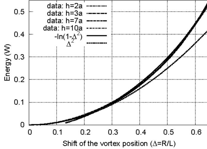
**Figure 2.** Energy of the vortex (15) vs. the vortex displacement  $\Delta$  from simulations on disks with the diameter  $2L = 40a$  and different thicknesses  $h$ ,  $\ell = 1.3a_0$ ,  $\alpha = 0.01$ .
