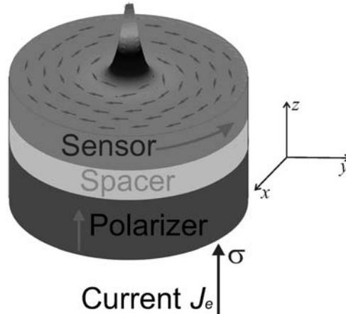
**Figure 1.** Schematic of the heterostructure.
