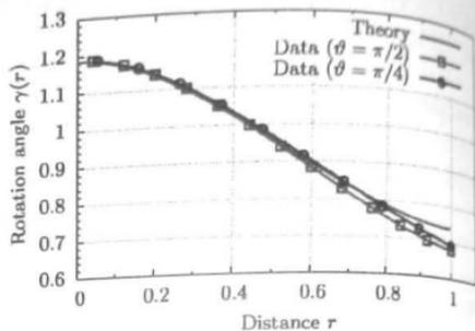
Fig. 2. Radial dependence of rotation angle  $\gamma$  in spherical particle. Line: numerical integration of (2). Symbols: SLaSi simulations for crystallographic directions [110] and [111]. Distance is normalized to sphere radius  $R$ .
