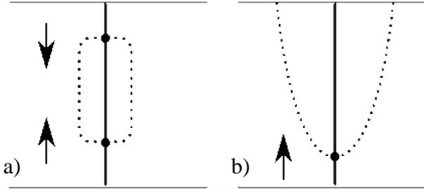
Fig. 1. Schematic of the BP dynamics during the switching under the action of DC field. (a) for exchange anisotropy simulations; (b) for dipolar ones. Solid curves indicate vortex lines, dotted curves correspond to the isosurface  $S_z = 0$ , circles indicate BP position, and arrows indicate BP motion direction.
