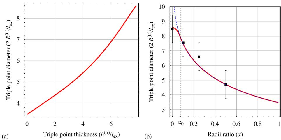
Fig. 8. The triple point analysis: the outer ring diameter as a function of (a) the ring thickness and (b) the radii ratio. Red lines correspond to the exact numerically calculated data (the local model of the magnetostatics), dashed blue line is the analytical solution (18), which is acceptable for  $\alpha > \alpha_0$ . Points with error bars were obtained from simulations data (Fig. 7).
