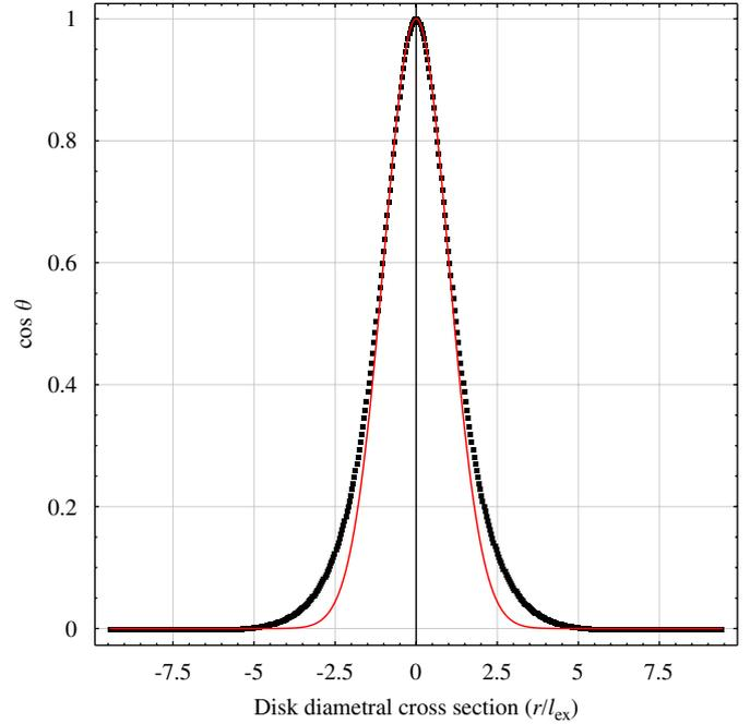
Fig. 2. The comparison of two OPV profiles: the ansatz (9) with  $\mu = 1$  and  $\lambda = \sqrt{2}$  (solid red line) and micromagnetic simulations (black bars) for the Py disk ( $R = 50$  nm,  $h = 5$  nm).
