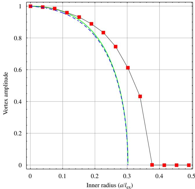
Fig. 4. Vortex amplitude (at the inner edge) vs. inner radius of the ring. Bars denote simulations results and solid green line corresponds to theoretical calculation, which were performed numerically. Dashed blue line corresponds to the fit (16). Other parameters are the same as in Fig. 2.
