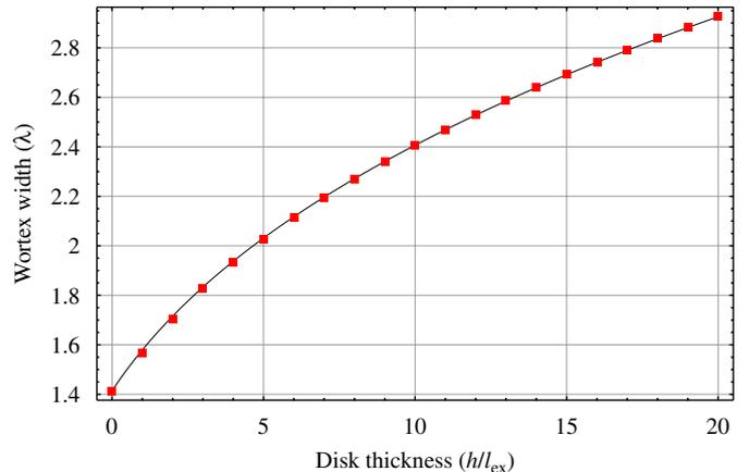
Fig. B3. The dependence of the vortex width in case of disk on disk thickness.
