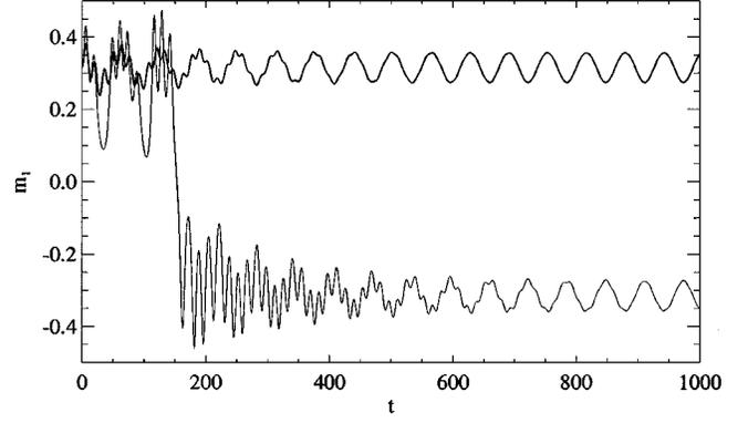
FIG. 3. Time evolution of the vortex core magnetization in the presence of the clockwise (upper curve) and counterclockwise (lower curve) rotating magnetic field based on Eqs (9). The parameters are  $A=a_1=a_2=b=1$ ,  $\mu_1=-0.1$ ,  $\omega=\pm 0.1$ ,  $h=0.0355$ ,  $\gamma=0.01$ . Initial polarization  $p=+1$ .
