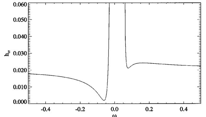
FIG. 4. Threshold value of the field amplitude  $h_{cr}$  versus  $\omega$ , as given by Eq. (11). The parameters used are  $a_1=b$ ,  $Ab/\alpha = 0.01$ ,  $\omega_0=0.08$ ,  $\gamma=0.002$ .
