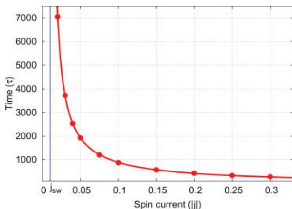
**FIGURE 9.** Switching time as a function of the applied current. [Color figure can be viewed in the online issue, which is available at [www.interscience.wiley.com](http://www.interscience.wiley.com).]
