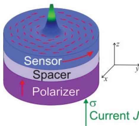
**FIGURE 4.** Schematic of the CPP heterostructure used for the current induced vortex dynamics. [Color figure can be viewed in the online issue, which is available at [www.interscience.wiley.com](http://www.interscience.wiley.com).]
